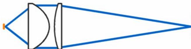
The space-angle product cannot be made smaller with discarding precious light. Furthermore, it cannot be arbitrarily increased without creation of optical aberrations that reduce contrast. The space-angle product must be skillfully managed for maximum collection of light.
